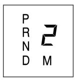
The tachometer display on the instrument panel cluster will show which gear the vehicle is in and a number indicating the requested gear range when moving the shift lever forward or rearward. See *Speedometer and Odometer on page 3-31* for more information on the odometer.
